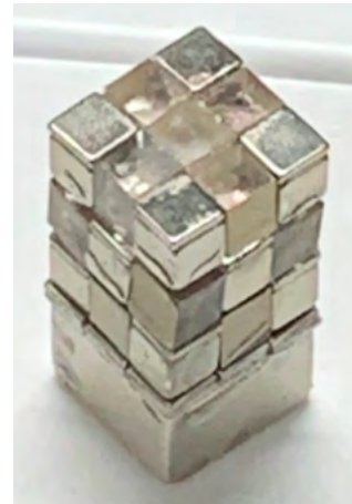
Fig. 3 Development of optimized magnet shape by combination of small magnets. The part where magnetic moment exists is formed by permanent magnets, and the part where magnetic moment does not exist is formed by acrylic.
